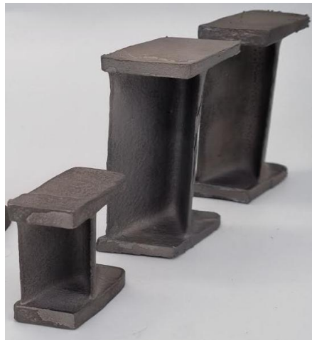
Figure 1 : NNS fully densified TiAl blades just after SPS sintering
